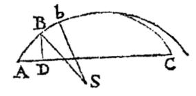
By *Lem.* 9 the force of the tension is to the absolute force in moving the element of length Bb is as BS to Bb. But the acceleration of the force is in the ratio composed directly from the absolute force and inversely as the matter to be moved. Whereby if the weight of the increment to be moved Bb is called p [we would call this mass rather than weight], the acceleration of the element Bb to the acceleration of the weight P arising from its own gravity, that is, the
