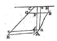
drawn crossing BF in G, then the total lateral pressure of the fluid, by which the surface AB has a force acting on it horizontally, is to the weight of the fluid enclosed in the space CABD, as the area AEGF is to the area CABD.
