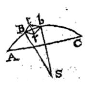
For a given density of a stretched string, the accelerating force at any point is as the curvature at that point.
