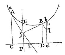
AB is part of a certain thin rope hanging from the points A and B; the normals AC and BD are drawn to the line with the given position CD parallel to the
