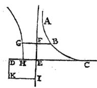
always FG = x = density of the rope at B. Then if GH is the curve, that always touches the point G, and the area GFEH of the end to the tangent CE is added to the area EDKI =  $\frac{a}{m}$ , the total area IKDHGFEI is always equal to the tension in the thread at B. For EF = y, and thus the fluxion of the area is yx = fluxion of the tension which is equal to  $\frac{a}{m}$  at the point C.
