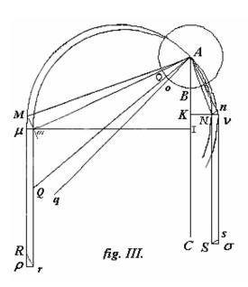
For if all the parts of the pulley are moving with the same velocity acquired from the height v, then the vis viva = Pv. Moreover since the parts which are closer to the centre are moving slower there, the vis viva is made smaller, as is made clear by computation.
