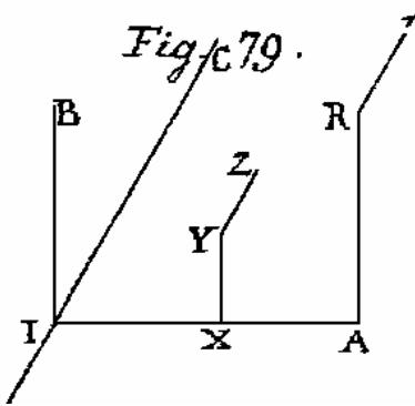
Hence the solution of the problem thus is reached: with a proposed axis of rotation  $IA$  of this kind, two directrices  $IB$  and  $IC$  are taken together (Fig. 79), so that for any element of the body  $dM$  with these parallel coordinates established  $IX = x$ ,  $XY = y$  and  $YZ = z$  and on putting  $XZ = \sqrt{(yy + zz)} = r$ , making  $\int xzdM = 0$ . Moreover on
