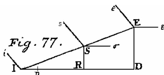
force can be resolved into two forces  $Ss$  and  $S\sigma$ , of which one  $Ss$  shall be in the plane normal to  $ID$ , and the other  $S\sigma$  now shall be parallel to the line  $ID$ .
