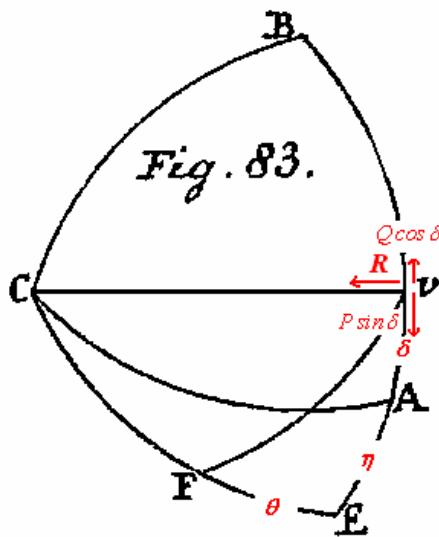
[Note that the components of the forces generating moments about the axis  $IF$  must be perpendicular to  $IF$ . This task is much simplified by considering the forces to act on the surface of a sphere as follows :]
