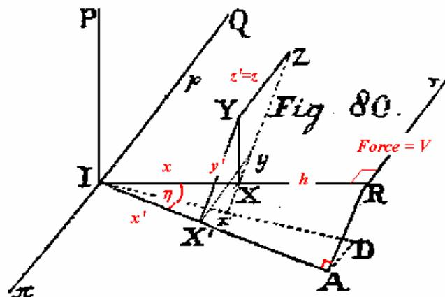
force  $V$ , thus so that it is normal to the plane of the diagram from the opposite side. From these two forces acting simultaneously, the body begins to rotate about some axis passing through the centre of inertia, and from the preceding paragraph it is apparent that this axis is placed in the plane of the diagram, which therefore shall be the axis  $IA$ , for which the position is required: thus putting the angle  $RIA = \eta$ , so that with the normal  $RA$  drawn from  $R$  to that
