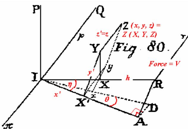
Let  $I$  be the centre of inertia of the body (Fig. 80), and in the diagram referred to as before, the plane through  $I$  is drawn normally to the direction of the force acting, which is  $Rr = V$ , in which there is put the distance  $IR = h$ . Then on
