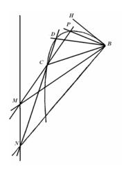
Therefore the meeting of the leg BH with the radius passing through the points C, D, P will delineate the section of the cone, and the right line BH tangent at the point B.
