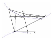
[Thus, the two methods of defining the conic section are shown, the first above using the parallelogram method, while the second below uses the idea of poles with an angle rotating about one pole and chords passing through the other pole from a variable point on a line.]
