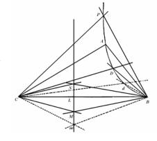
cone passing through the points B and C; and when the point m approaches towards the points L, M, N, the point d (by construction) will approach towards the points A, D, P. And therefore the conical section passes through the five points A, B, C, P, D.
