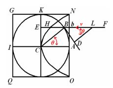
particle of the medium, by being incident obliquely along the right line FB, strikes the sphere at B, will be to the force by which the particle may strike the same cylinder ONGQ at b, with the axis ACI described perpendicularly around the sphere, as LD to LB or as BE to BC
