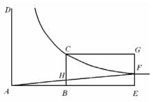
CBEF shown by the hyperbolic area, and the motion of this at the end of the time may be shown by the ordinate EF of the hyperbola, with the part of its motion EG lost. And the resistance of this at the end of any time may be expressed by the length BH, with the part CH lost to resistance. All these are apparent by Corol.1.& 3, Prop. V. Book II.
