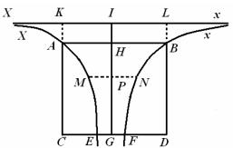
indefinitely to the parts X, x; truly the figure EMAHG will be generated, that part of the cataract which is contained within the vessel ABDC.
