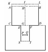
Now the openings of the pipe *EF* and *ST* may be closed, and the small circle may ascend in the fluid compressed on all sides and by itself ascending it may force the water above to fall through the annular space between the small circle and the side
